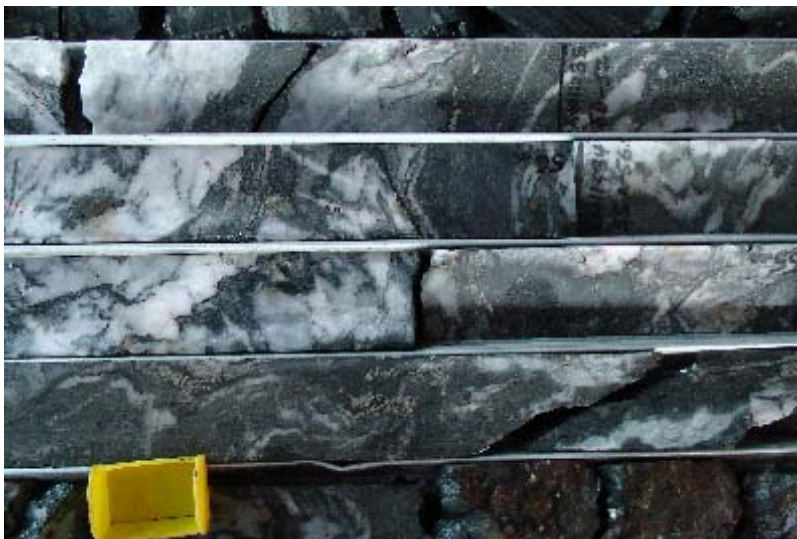
Bepkong core showing deformed sediments, alteration, veining and sulphides. Source: Author
